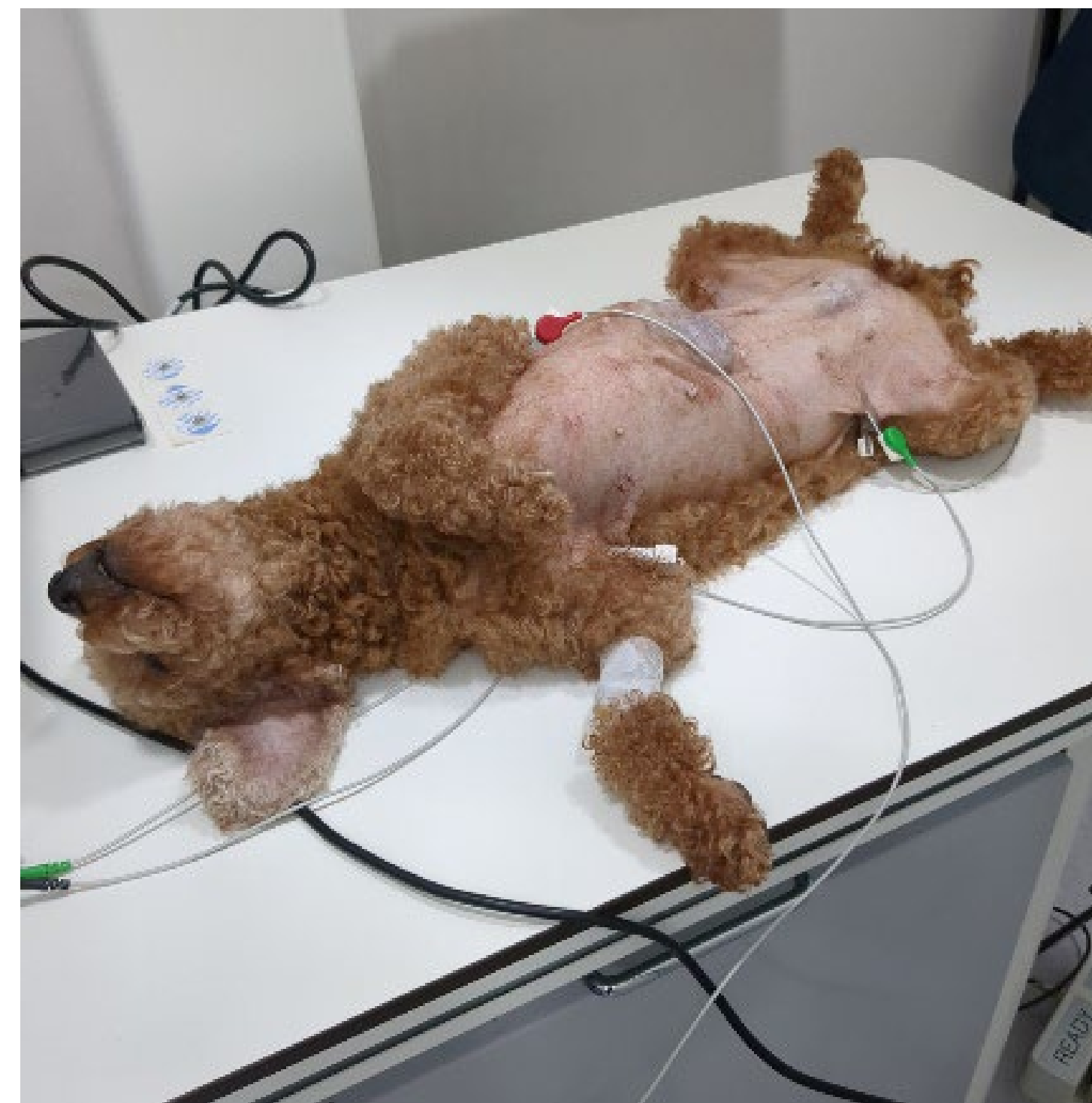
Verify reliability by comparing ECG on anesthetized dogs with non-contact measurements
