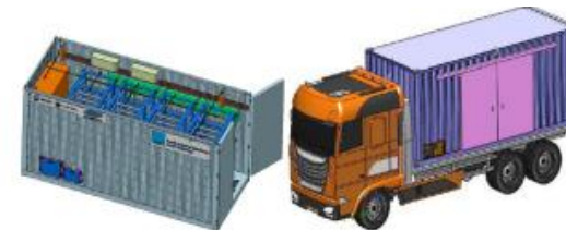
Fig. 4. Concept of removable battery truck.
